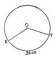
In the diagram, O is the centre of the circle, radius 14 cm. If the length of the minor arc XY is 36 cm, calculate the area of the minor sector OXY. [ Take  $\pi = \frac{22}{7}$ ].
